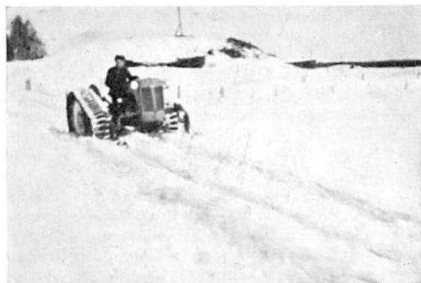
Fig. 4. Tractor equipped with rubber tracks and runners making its own road. — The worst obstacles are cleared during the summer. In the winter the snow is »packed» with tractor and drag. The only road maintenance carried out is dragging. — Photo Metsäteho
